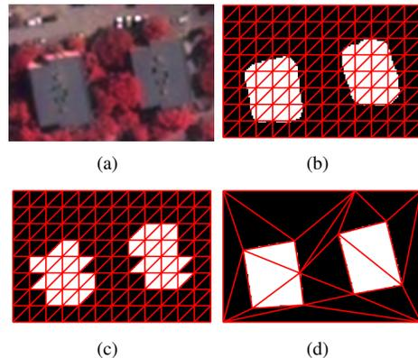
**Fig. 1.** Input image and example labeled meshes. (a) Input image, (b) Initial fine lattice, (c) Initial and (d) Optimized labeled triangle meshes. The triangles labeled as building are indicated by white.
