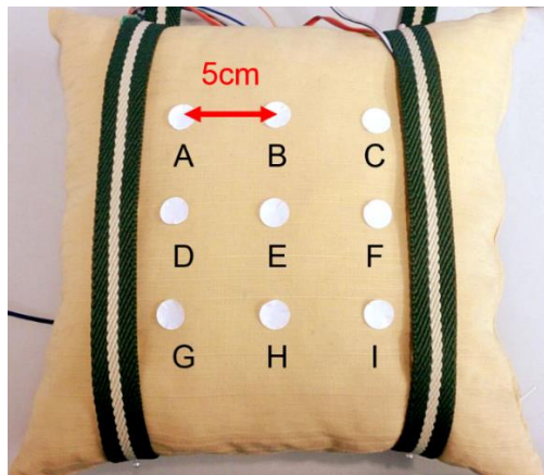
Fig. 6. Arrangement of markers on a cushion.
