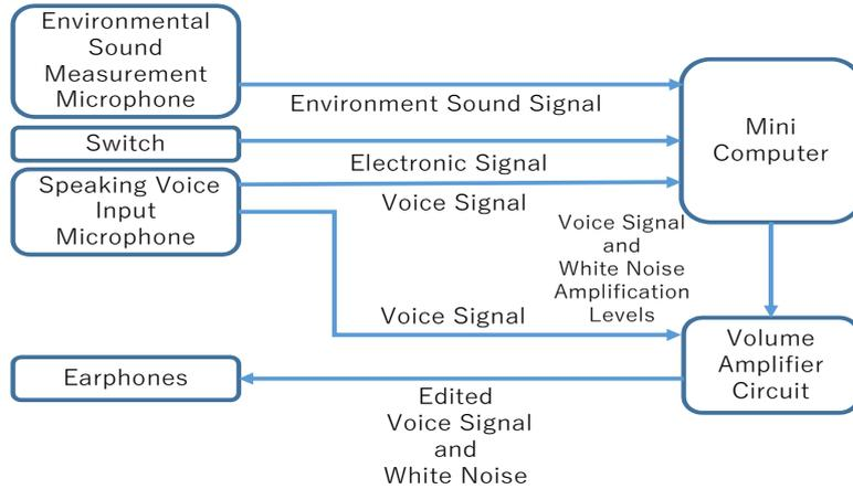
Fig. 1. System configuration
