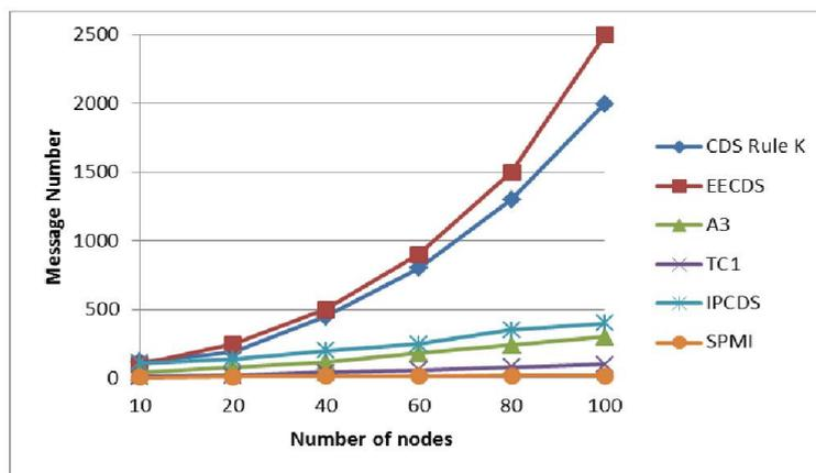
Fig.4. Message overhead versus network size
