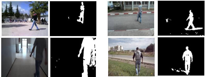
Fig. 2. Background subtraction results in personnel video database in both indoor and outdoor environments
