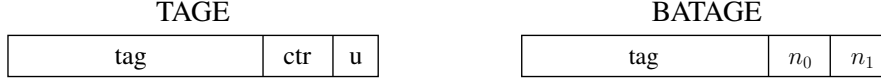
Figure 4: Tagged entry in TAGE (left) vs. BATAGE (right). The payload of a TAGE entry consists of an up/down counter (typically, 3 bits) and a u counter (1 or 2 bits). The payload of a BATAGE entry consists of two counters n_1 and n_0 (typically, 3 bits each) counting respectively the number of taken and not-taken occurrences.
