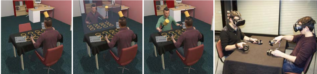
Figure 1: Setup of the experiment: each user was able to interact in the virtual environment with his own avatar, while the physical setup provided both a reference frame and passive haptic feedback. From left to right: experimental conditions Alone, Mirror and Shared; Physical setup of the experiment.
