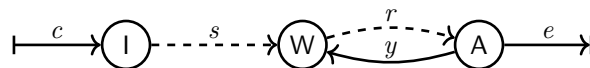
Fig. 1. Example resource automaton for request handlers. Dashed arrows \dashrightarrow denote controllable transitions; \dashleftarrow (resp. \dashrightarrow ) denote resource appearance (resp. disposal).
