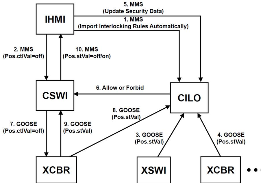
Figure 1. IEC 61850 CILO-controlled switchgear operation [8].
