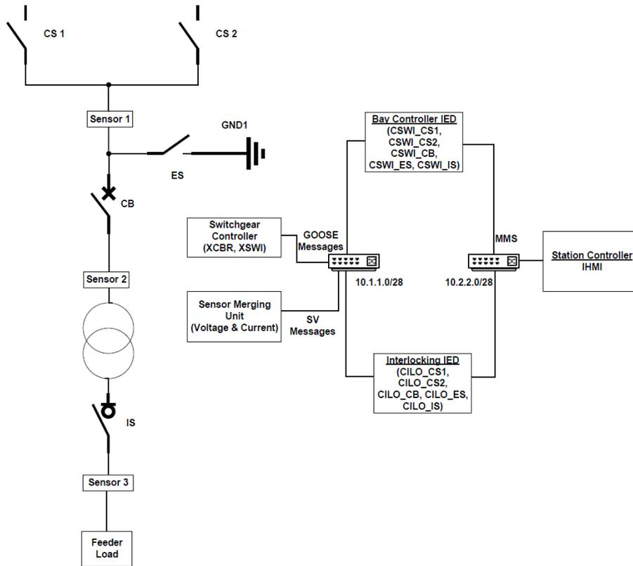
Figure 3. Implementation schematics of the substation testbed.
