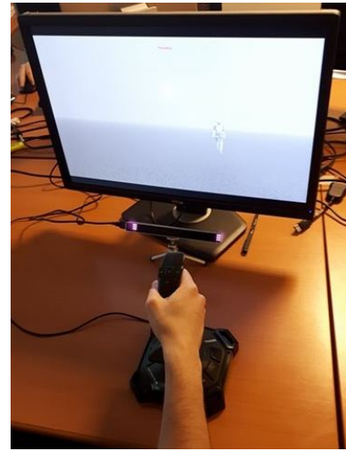
Figure 1: Example of a participant during our experiment. Participants are seated in front of a 24-inch screen. They use a joystick to navigate in the virtual environment and to avoid a virtual walker. An eye-tracker is located below the screen and records their eye movements.
