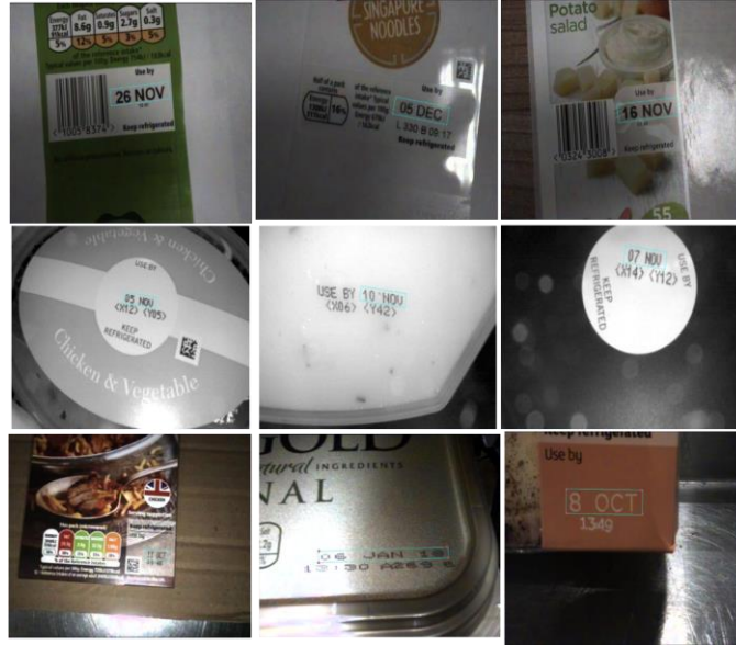
Fig.7. FCN detection results of the date code on different packages.
