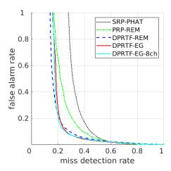
Fig. 3: ROC curve for the LOCATA dataset.
