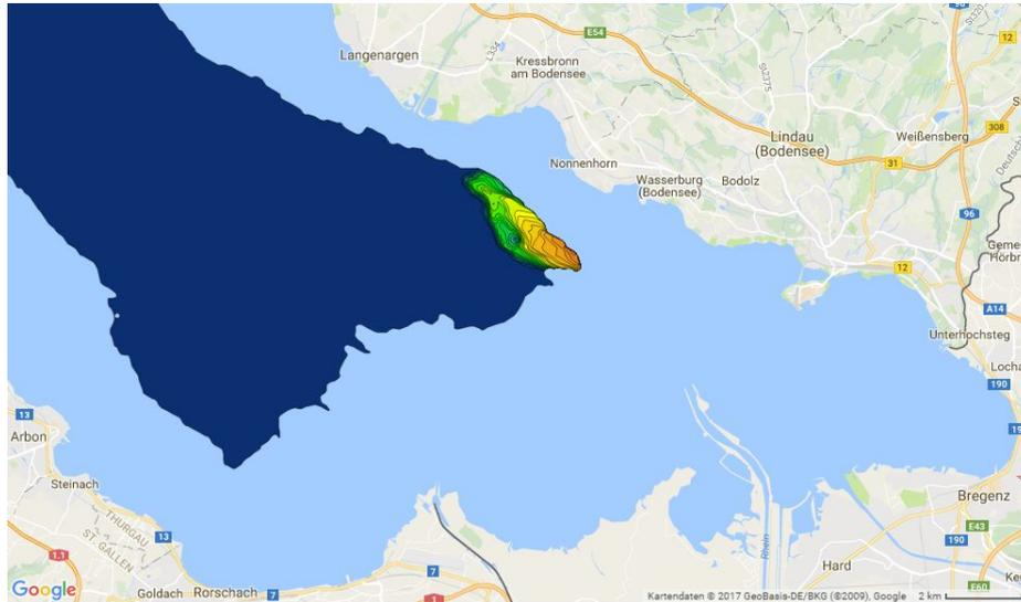
Fig. 1. 2D slice at 140m water depth visualizing suspended sediment concentration
