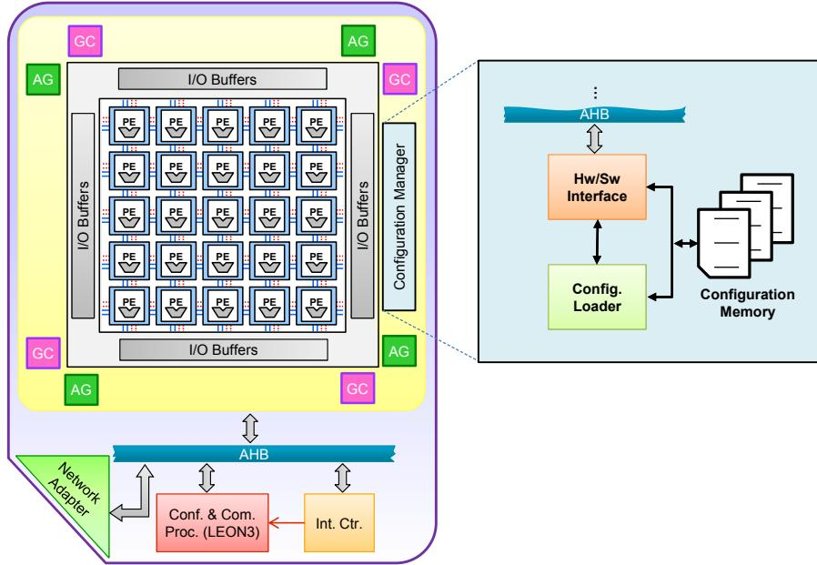
**Fig. 1.** An abstract architectural view of a TCPA is shown on the left. The abbreviations AG and GC stand for address generator and global controller, respectively. On the right side is the configuration manager (CM) shown that provides the interface to reconfigure the entire TCPA architecture.
