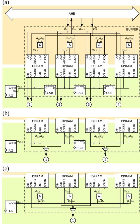
**Fig. 2.** In (a), (b), and (c), a reconfigurable I/O buffer architecture is shown which may be configured into different modes and trade-off the buffer sizes with the number of available independent ports to the processor array [3].
