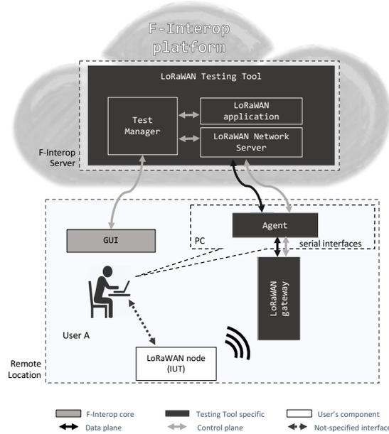
Fig. 4. LoRaWAN remote interoperability test set up.
