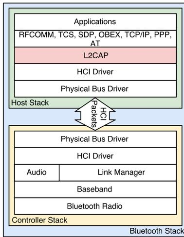
**Figure 1: Bluetooth stack and the L2CAP layer.**
