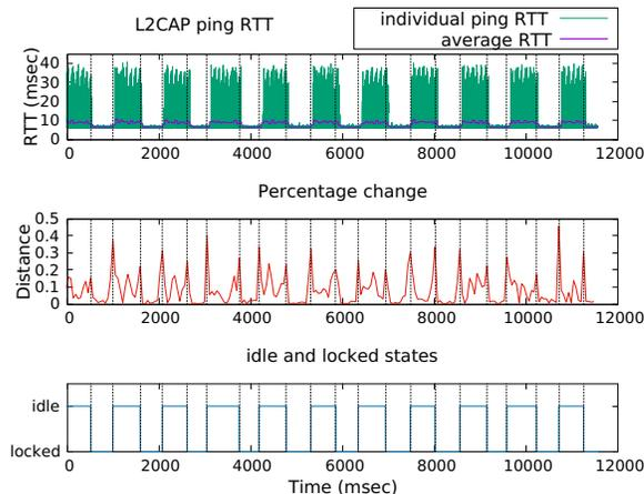
**Figure 2: Bluetooth ping flood RTTs (individual and average), percentage change and actual state (ground truth) while alternating between *idle* and *locked* states. The percentage change is computed from the average RTTs. Vertical bars correspond to the times of the actual state changes.**
