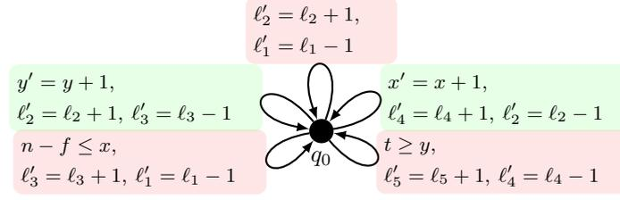
■ **Figure 6** A counter automaton for the threshold automaton in Figure 1.
