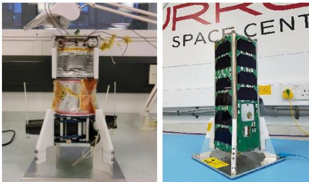
**Figure 11. Left: The complete InflateSail Payload Showing the CFRP Booms (bottom), the Z-Folded Sail Membrane (middle) and the Origami Folded Inflatable Mast with CGGs (top); Right: The integrated InflateSail CubeSat**
