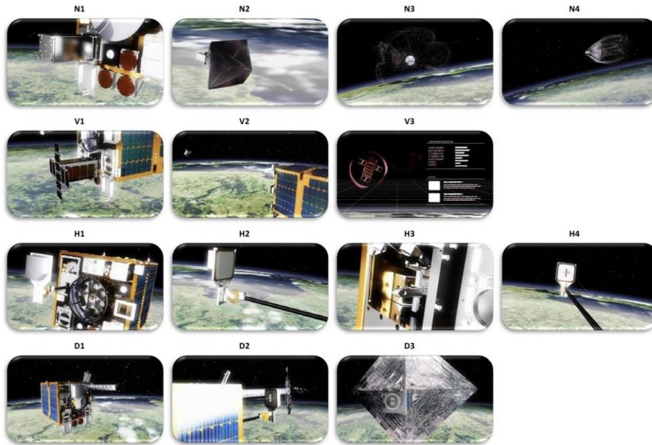
**Figure 2. N1 to N4: net experiment, V1 to V3: vision-based navigation experiment, H1 to H4: harpoon experiment, D1 to D3: dragsail experiment.**
