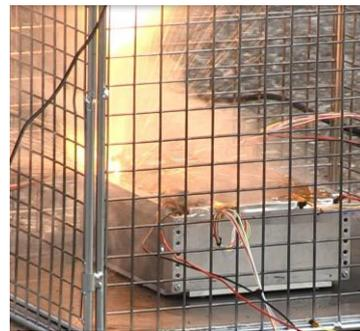
**Figure 13. Test Battery induced into thermal runaway**
