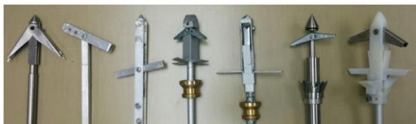
**Figure 9. Harpoon projectile prototypes and evolution.**
