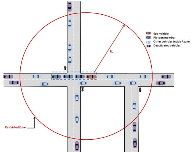
Fig. 3. Restricted Zone of transmission for platoon communications
