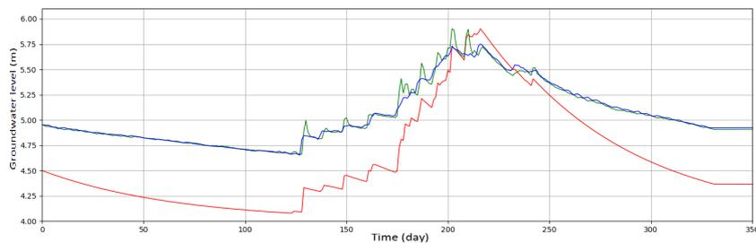
Figure 2 : Forecast realized by (hydraulic model + adjustment module) in Green, Observations in Blue and Forecast realized by model without adjustment module in red
