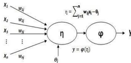
**Figure 2.** Representation of an artificial neuron [4]. Inputs are multiplied by their weight. The products are added to give the weighted sum. The threshold of the node is subtracted from the weighted sum to determine the output of the node.
