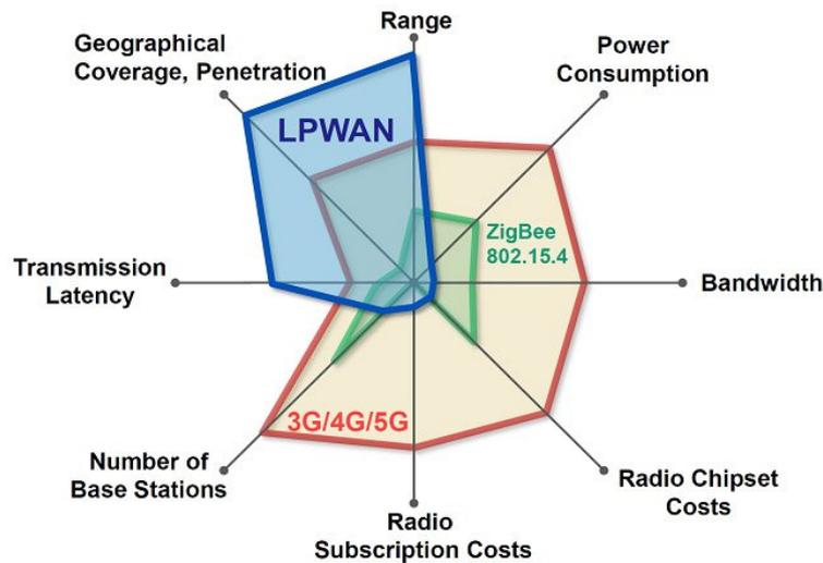
**Figure 4.** comparative communicating technology of 100 bps.
