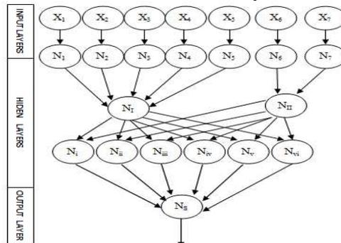
**Figure 3.** Architecture of the neural network. The variables  $X_1 \dots X_7$  represent the morphological and frequency properties, respectively the negative form, the maximum amplitude, the minimum amplitude, the maximum width, the minimum width, the hearth rate and the hearthbeat. The variables  $N_1 \dots N_{vi}$  represent the intermediate nodes. The Node  $N_8$  determines the arrhythmia type.
