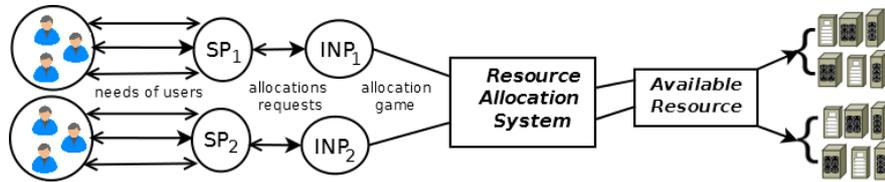
Figure 2 – Ressource allocation process.
