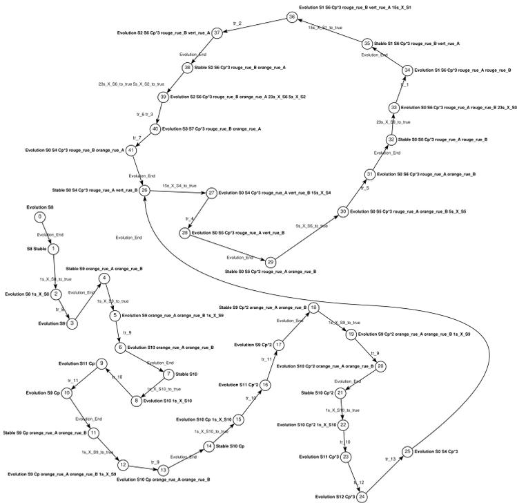
Figure 3. Automaton based on algorithm 1 (stable and unstable states of the grafcet)
