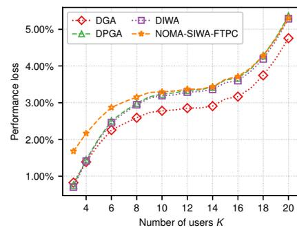
Fig. 4. Performance loss vs. different number of users,  $M = 2$
