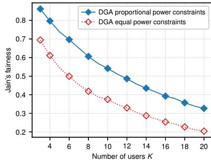
Fig. 12. Fairness index vs. different number of users,  $M = 2$
