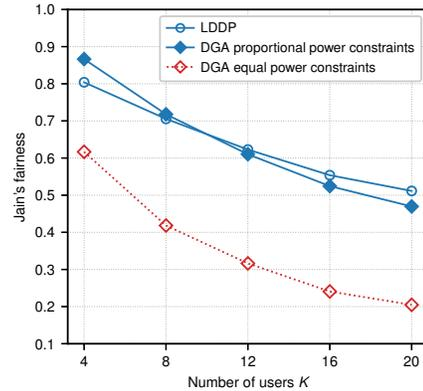
Fig. 14. Fairness index over a scheduling frame,  $M = 2$
