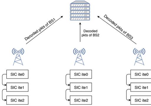
Fig. 2: Algorithm of local SIC at each BS. The BSs perform SIC locally, then forward their decoded packets to the back-haul. *It*<sub>0</sub> represents the procedure of a simple receiver; the maximum SIC iteration is defined to 2.
