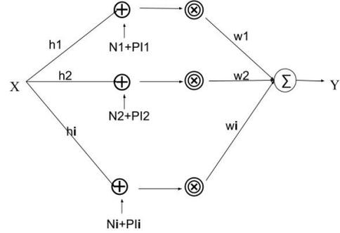
Fig. 1: Algorithm of SC/MRC/EGC.  $x = \pm 1$  represents the transmitted symbol,  $h_i$  is the channel gain of BS $_i$ ,  $N_i$  and  $P_i$  are the noise and the interference experienced by the expected signal in the branch BS $_i$ ,  $w_i$  is the weight at the  $i$ th branch.
