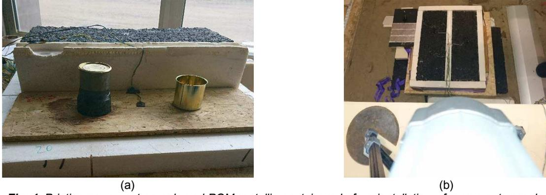
**Fig. 1.** Pristine pavement sample and PCM metallic containers before installation of pavement sample with voids with T-type thermocouples (a) and pavements samples with FLIR A320G infrared camera (b)
