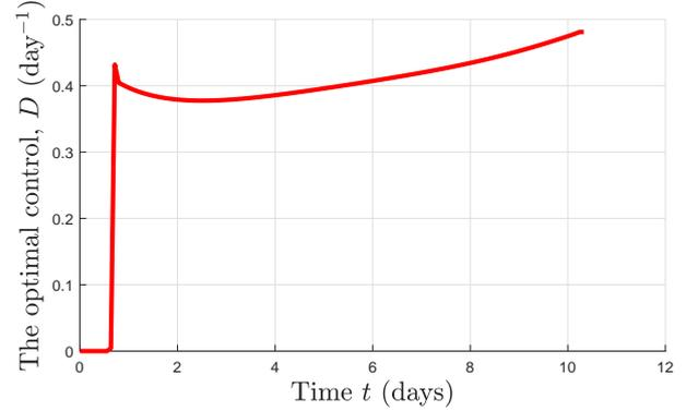
Fig. 2. The optimal control provided by Bocop when  $s^0 = 1 > s_c$  is a *bang(0)-singular* control law.
