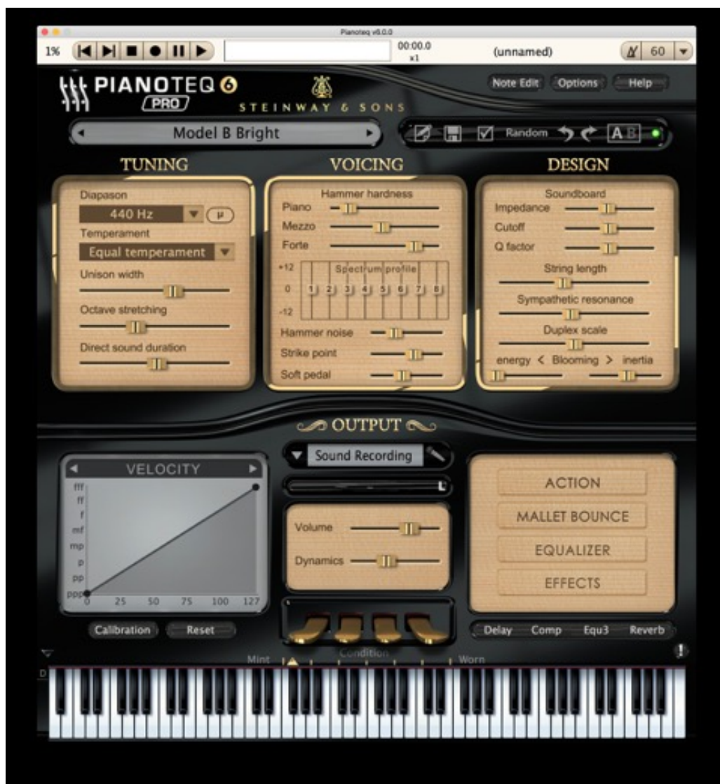
Figure 7: Pianoteq PRO 6 interface. The Pianoteq software computes the piano sound in real time using physical models.
