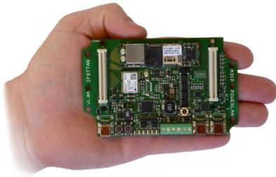
Figure 9: Generic wireless sensor platform PEGASE 2
