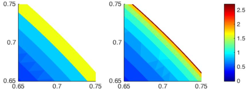
FIGURE 5.3. Logarithm of the norm of the gradient of the discrete solutions to the first example in §5.2 for  $s = 0.6$  using uniform (left) and graded (right) meshes with approximately the same number of degrees of freedom (12636 and 12656, respectively). The pictures correspond to a zoom on the square  $[0.65, 0.75]^2$ .
