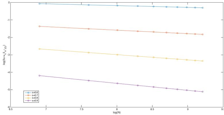
FIGURE 5.1. Errors for the first example described in §5.1. Least squares fitting of the data yields estimated orders of convergence 0.101 for  $s = 0.6$ , 0.200 for  $s = 0.7$ , 0.301 for  $s = 0.8$ , and 0.402 for  $s = 0.9$ .
