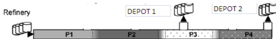
Fig.1. Single unidirectional multiproduct pipeline system
