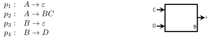
Figure 1. A grammar for a role that provides a service A and uses the external services C and D . B is an internal task, bound to the role, and whose name can henceforth be changed.
