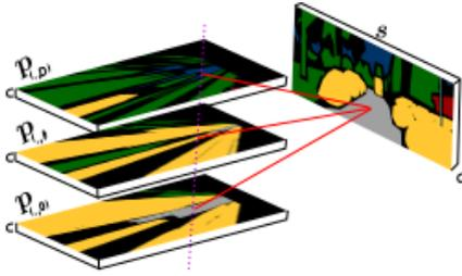
Fig. 3: A sample transformation of the projective semantic information into the planes that are parallel to the occupancy grid is shown.  $C$  represents the number of classes. The class probability values are colored for illustration purposes.
