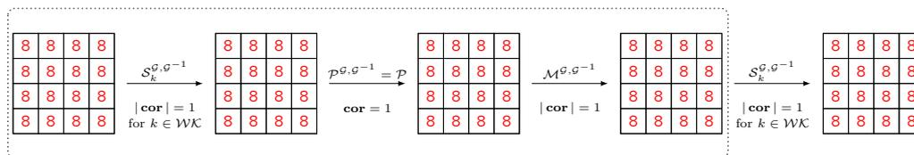
**Figure 1:** The  $\mathcal{G}$ -shifted linear trail for one round of Midori64 corresponding to the invariant attack.  $\mathcal{G} = (G, G, \dots, G)$  is any permutation for which  $\langle 8, G(x) \rangle$  is equal to the invariant  $g(x) = x_3x_2 + x_2 + x_1 + x_0$  for the S-box. In this trail, all S-boxes are active.
