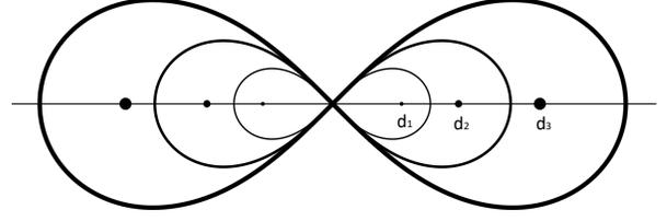
Fig. 4: Different Movement intensities and targets motion used in user study 2: Lemniscates of Bernoulli with half focal distances  $d_1(40^\circ) < d_2(100^\circ) < d_3(160^\circ)$ . The path of the targets lays in a sphere centered on the user.
