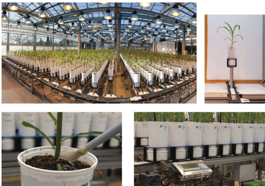
Figure 1 The Phenoarch phenotyping platform is one of the Phenome node in Montpellier. It has a capacity of 1,500 plants per experiment with a controlled environment (e.g., temperature, humidity, irrigation) and automatic imaging through time (13 images per plant per day).
