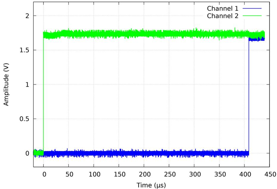
**Fig. 3.** Signals are desynchronized. Channel 1 for GPIO signal sent by core 1, channel 2 for GPIO signal sent by core 2. Time span between the two rising edges is due to “ $x * desynch\_value + x$ ” in 1.3.
