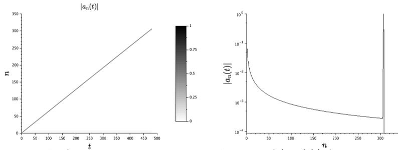
FIGURE 4. Left plot : space time evolution of  $|a_n(t)|$  for system (4) with  $p$  large, free-end boundary conditions and an initial condition localized on the first particle ( $a_1(0) = -i$ ,  $a_n(0) = 0$  for  $n \geq 2$ ). We have fixed  $p = 201$  in the numerical simulation. One observes a solitary wave with velocity  $v \approx 0.63 \approx 2/\pi$ . Right plot : spatial profile of  $|a_n(t)|$  at  $t = 479.84$  (semi-logarithmic scale).
