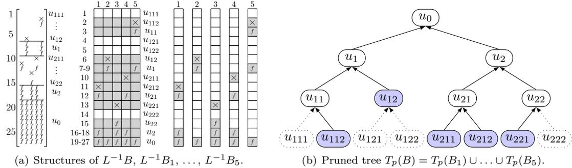
FIGURE 2. Illustration of multiple RHS and tree pruning.  $\times$  corresponds to an initial nonzero in  $B$  and  $f$  to “fill-in” that appears in  $L^{-1}B$ , represented in terms of original variables and tree nodes. Gray parts of  $L^{-1}B$  (resp. of  $L^{-1}B_i$ ) are the ones involving computations when RHS columns are processed in one shot (resp. one by one).
