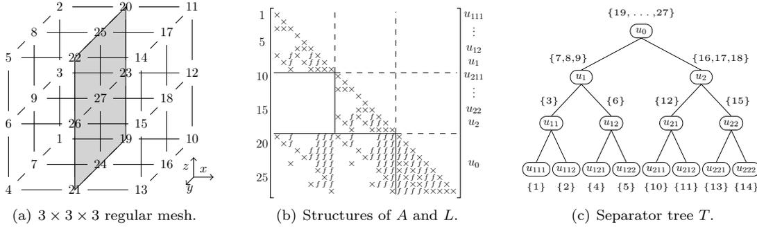
FIGURE 1. (a) A 3D mesh with a 7-point stencil. Mesh nodes are numbered according to a nested dissection ordering. (b) Corresponding matrix with initial nonzeros ( $\times$ ) in the lower triangular part of a symmetric matrix  $A$  and fill-in ( $f$ ) in the  $L$  factor. (c) Separator tree, also showing the sets of variables to be eliminated at each node.
