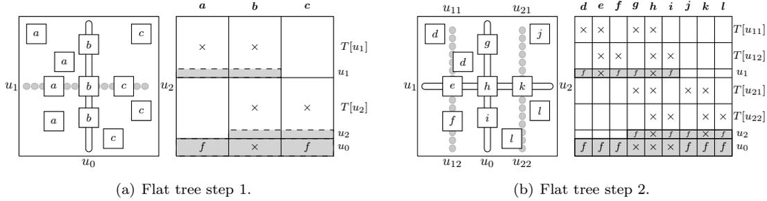
FIGURE 5. *Flat tree geometrical illustration.* In (a) and (b), the figure on the left represents different types of RHS, and the one on the right the permuted RHS matrix.  $\times$  or  $f$  in a rectangle indicate the presence of nonzeros in the corresponding submatrix, parts of the matrix filled in gray are fully dense and blank parts only contain zeros.
