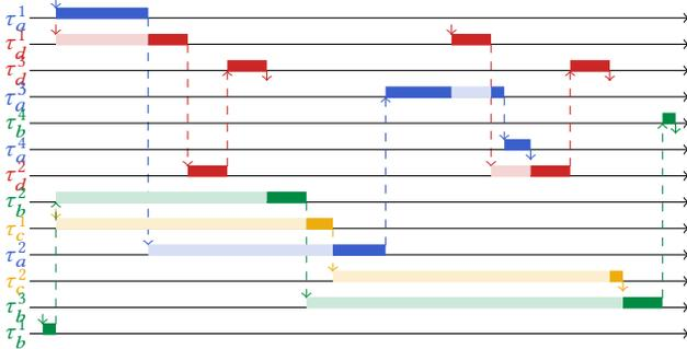
**Figure 1: A system with four task chains. Task priorities are decreasing from top to bottom.**
