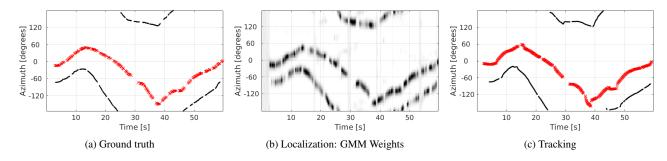
Figure 2: Results of speaker localization and tracking for Recording #1 / Task #6. (a) Ground truth trajectory and voice activity (red for speaker 1, black for speaker 2). Intervals in the trajectories are speaking pauses. (b) Result for localization, i.e. GMM Weights. (f) Result for tracker. Black and red colors demonstrate a succesful tracking, i.e. continuity of the tracks despite of speech pauses.
