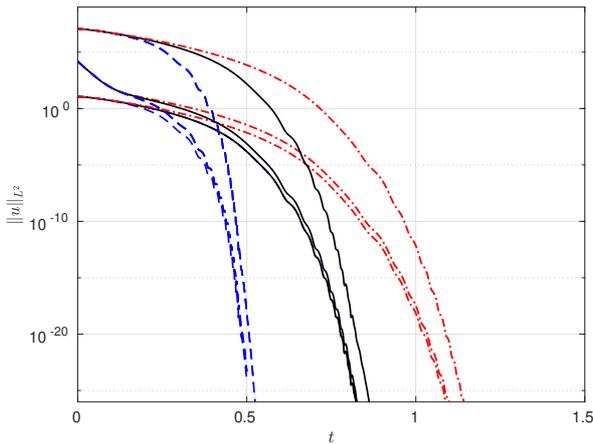
Figure 4. Evolution of the  $L^2$ -norm of the closed-loop system (logarithmic scale) with time-varying feedbacks for different initial conditions and prescribed times:  $T = 0.6$  (blue dashed line),  $T = 1$  (black line) and  $T = 1.5$  (red dotted dashed line) .
