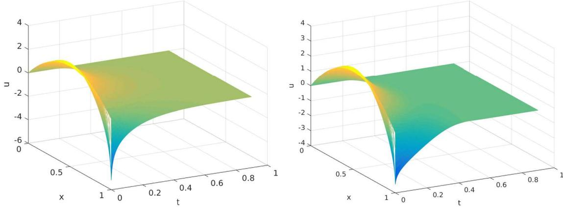
Figure 1. Numerical solution of the closed-loop system with boundary controller  $U$  (whose kernel gain is (33)) for exponential stabilization (left) and boundary time-varying controller  $U$  (whose kernel gain is (32)) for fixed-time stabilization with prescribed time  $T = 1$  (right).
