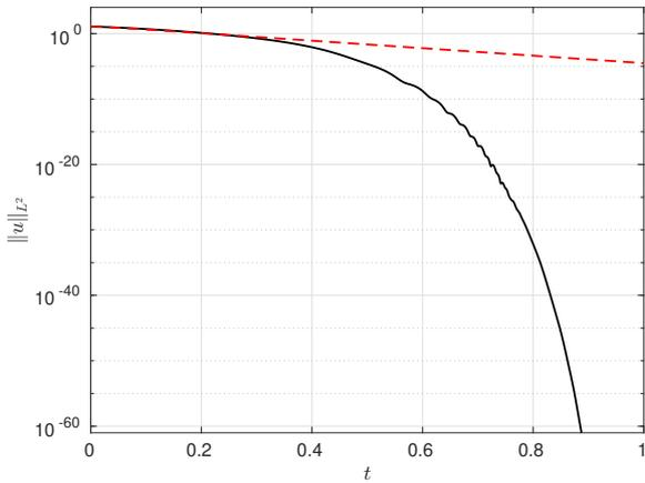
Figure 2. Evolution of the  $L^2$ -norm of the closed-loop system (logarithmic scale) with time-varying feedback (black line) for a prescribed time  $T = 1$  and linear control feedback (red dashed line) for exponential stabilization.
