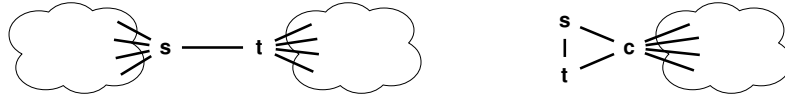
Fig. 1. Left: connected graph with one st -cut. Right: 2-edge-connected graph with two st -cuts. The clouds correspond to cliques.
