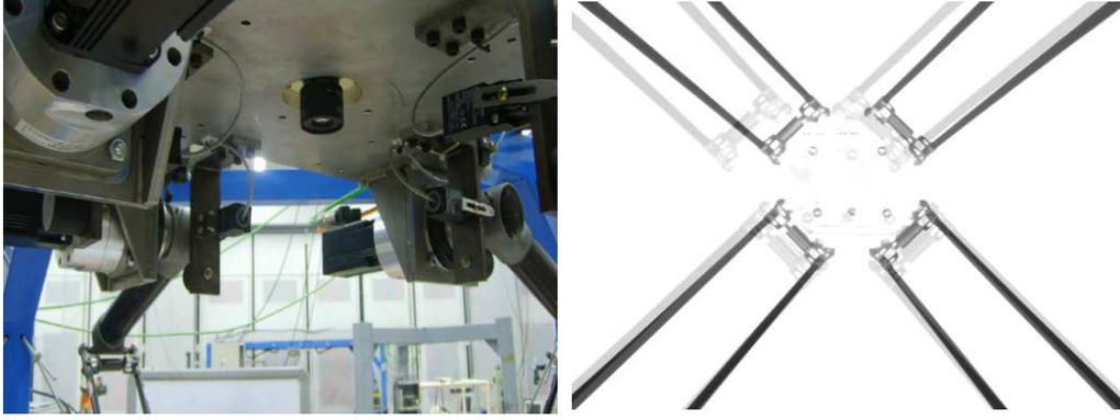
Fig. 14. A photograph of the Par4 robot (left) and a current configuration seen from the camera (the desired configuration is in the background).
