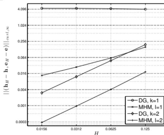
Standing wave in a PEC cavity: comparison between the MHM method and the DG method with respect to the  $\|(\mathbf{H} - \mathbf{H}_H, \mathbf{E} - \mathbf{E}_H)\|_\infty$  (left) and  $\|(\mathbf{H} - \mathbf{H}_H, \mathbf{E} - \mathbf{E}_H)\|_{\text{cur}1, \infty}$  (right) norms.
