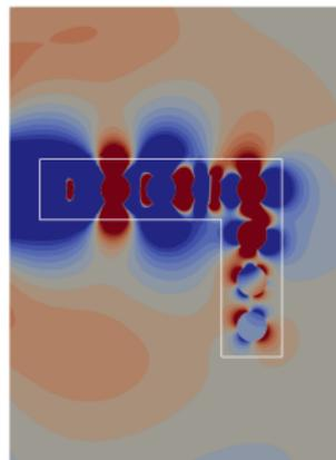
L-shaped waveguide formed of seven 50 nm diameter Au spheres in vacuum, with a 75 nm center-to-center spacing (computational domain: 550 nm  $\times$  750 nm  $\times$  400 nm).
