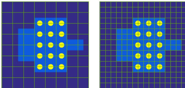
Nanowaveguide problem: coarse quadrangular meshes
