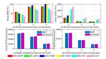
Fig. 8. Protocols' Performance with Grid Topology (Gateway at Network Center)
