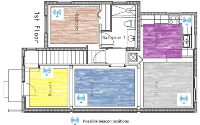
Fig. 5: An example of a beacon topology in a house. With different colors are the areas where the Beacon Setup application user should walk for half a minute in order to create the signal fingerprint for each room.
