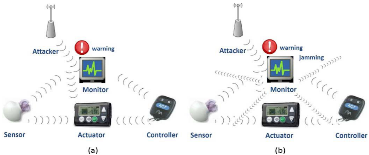
Fig. 4. MedMon working mechanism [10]
