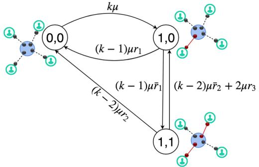
Figure 1: CTMC for a system with at least three links and buffer size one for each link.  $k$  is the number of links,  $\mu$  is the rate of entanglement generation, and  $r_1$ ,  $r_2$ , and  $r_3$  are parameters that specify the scheduling policy.
