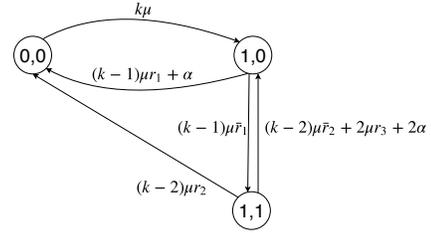
Figure 7: CTMC for a system with at least three links and buffer size one.  $k$  is the number of links,  $\mu$  is the rate of entanglement generation,  $\alpha$  is the decoherence rate, and  $r_1, r_2, r_3$  are parameters that specify the scheduling policy.
