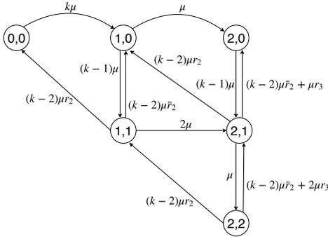
Figure 4: CTMC for a system with at least three links and buffer size two for each link.  $k$  is the number of links,  $\mu$  is the rate of entanglement generation, and  $r_2$  and  $r_3$  are parameters that specify the scheduling policy.
