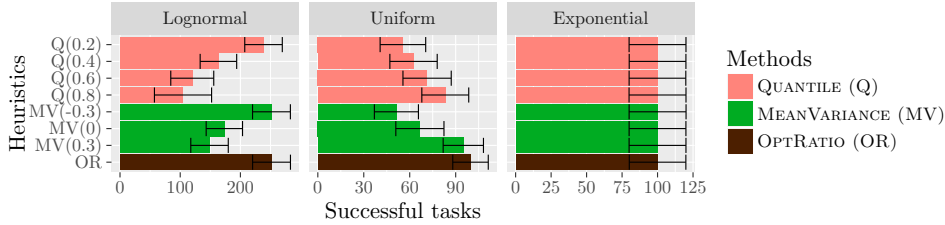
Figure 2: Number of successfully executed tasks for each heuristic with three distributions (lognormal, uniform, exponential) of same expected value \mu = 1 , with a budget and deadline b = d = 100 (which means that a single machine is enrolled). Each heuristic is run 100,000 times for each scenario. The error bars are computed with the mean plus/minus two standard deviations of the number of successes. The lognormal distribution has parameters \alpha \approx -1.15 and \beta \approx 1.52 to have an expected value \mu = 1 and a standard deviation \sigma = 3 , and the optimal cutting threshold for OPTRATIO is l \approx 0.1 ). The exponential distribution has shape \lambda = 1 and the cutting threshold is arbitrarily set to l = 2 . The uniform distribution has parameters a = 0 and b = 2 , and the cutting threshold is l = 2 .
