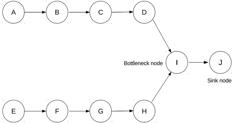
Figure 3: Canonical topology used in the simulation campaign. All non-root nodes periodically send packets to Node J. Exact simulation parameters are listed in Table 1.
