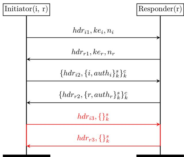
Fig. 6. The IKEv2-Sig-conf protocol. We add the key confirmation exchange. Connections are installed only after this exchange.
