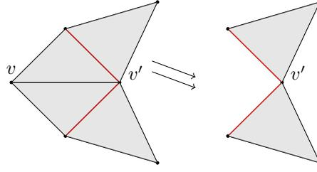
■ **Figure 1** Illustration of an *elementary strong collapse*. In the complex on the left,  $v$  is dominated by  $v'$ . The link of  $v$  is highlighted in red. Removing  $v$  leads to the complex on the right.
